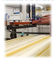
With its unique application of laser technology, the Wood-Runner is capable of accuracy to within one thirty- second of an inch. No other automated lumber retrieval system utilizes this application of laser technology or achieves this level of accuracy.
